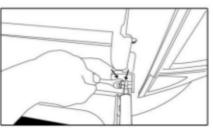
place rod end of damper and tigten back bolt A
