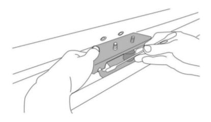
3.install tailgate lift set to replace the original bracket using original bolts
