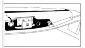
place the bracket of the damper and tighten bolt A back
