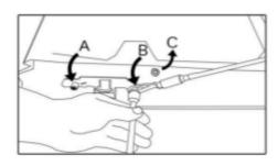
un-bolt bolt A and B take out flat washer C
