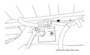
6.attached the bracket to the trunk using original btacket and nuts.
