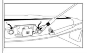
put sling back in place and tighten bolt B
