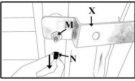
5.2 put main bracket (X) in position. Finger tighten nut M
