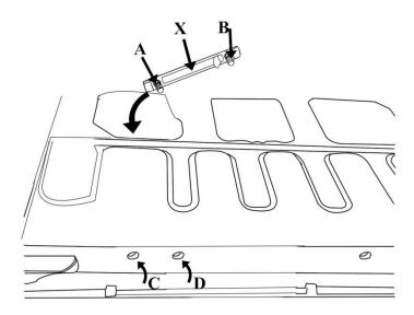
2. put bracket X into the tailgate (peel off glue tape and stick it inside the tailgate). Place bolt A&B through hole C&D
