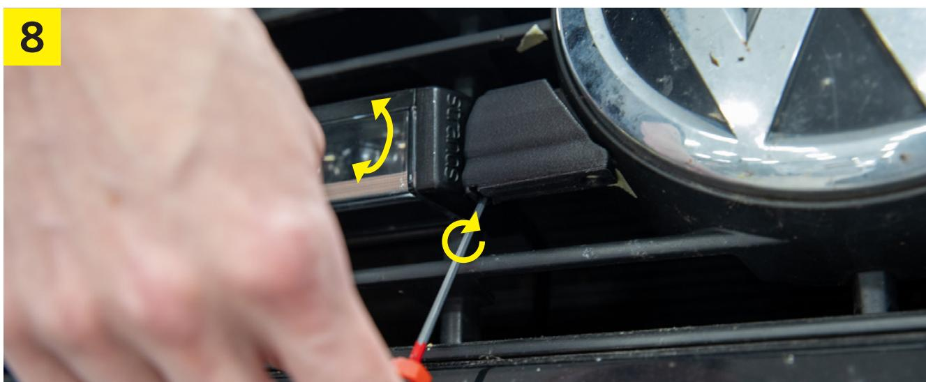
Adjust the angle of the light bar, then tighten the screw on the underside of the center bracket to lock the bar in place. Repeat all steps on the other side.
