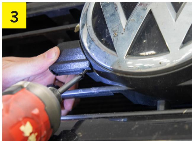
Fasten the bracket using the supplied screw.
