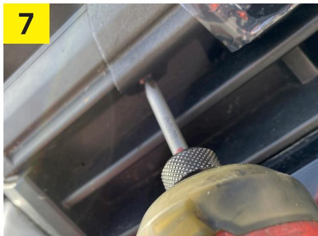
Fasten the side bracket using the supplied plastic screws. Push the light bar and bracket toward the center before tightening the screws.
