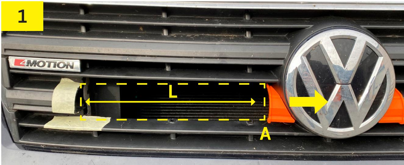
Carefully cut an opening in the grille to fit the LED bar.
