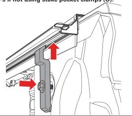
Place the outer part of the clamp (O) into the stake pocket, up underneath the plastic bed cap, then secure to the bolt. Make sure the rail is level. Tighten all clamps to 10 ft/lbs of torque with a 1/2" wrench or socket. Caution: Do NOT overtighten! Repeat steps 5-8a on the opposite side with the driver's side rail (B).
