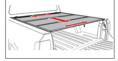
Check if the latches are hitting or not engaging the side rails (A & B) by releaseing each latch. If any of the latches need modifications, refer to the Slam Latch Adjustment section on the next page on how to make adjustments.
