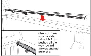
Attach two clamps (G) from the passenger side rail (B) to the truck bed. Place the front clamp 6-8 inches from the bulkhead. Place the center clamp to the rear of the prop rod. For the best cover fit, the side rails (A & B) should be level with the truck bed cap and not angled up or down.
