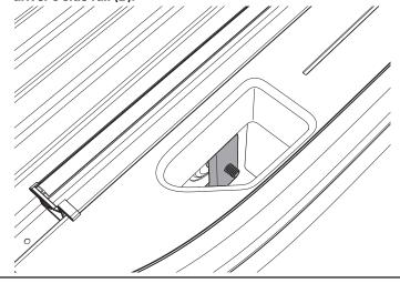
FOR 07-13 SILVERADO/SIERRA APPLICATIONS ONLY Install a stake pocket cover (P) near the tailgate where the stake pocket is on both sides of the bed as shown.
