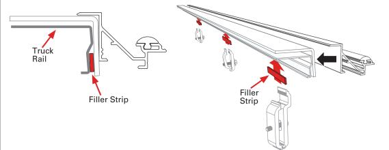
IMPORTANT: In order for the cover (C) to operate properly the side rails (A & B) MUST be square (90° angle) to the truck bed rails. This allows the rear latch to engage properly.
