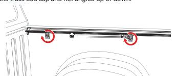
**NOTE**: For steps 5-8a: If the rails are leaning down, have one person stand on the outside of the bed and slightly roll the rails upward while another person slowly snugs the clamps up. If the clamps are tightened too quickly or overtightened, it will cause the rails to lean down.
