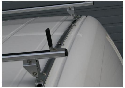
Minimum weight with maximum strength in aerodynamic design. The mounting system allows a flexible position on the roof. The crossbars were developed for a maximum total load of 150 kg (the maximum roof load restrictions by the vehicle manufacturer must be observed anyway). For VW Crafter 35 with long wheelbase, high roof with factory channel. Dimensions: wheelbase 4325 cm, complete hight 2705-2755cm, complete length 6940 cm .
