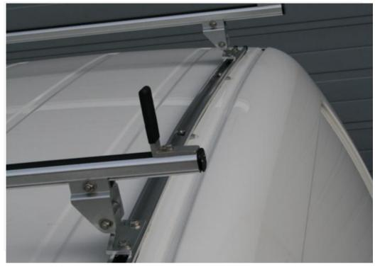
Minimum weight with maximum strength in aerodynamic design. The mounting system allows a flexible position on the roof. The crossbars were developed for a maximum total load of 150 kg (the maximum roof load restrictions by the vehicle manufacturer must be observed anyway). For VW Crafter 30 and 35 with medium wheelbase, high roof without factory channel. Dimensions: wheelbase 3665 cm, complete hight 2705-2755 cm, complete length 5905 cm.
