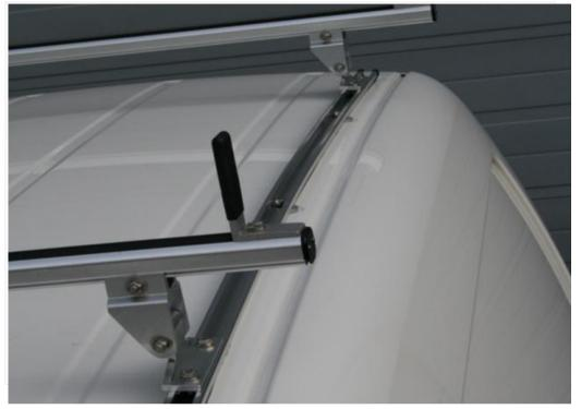
Minimum weight with maximum strength in aerodynamic design. The mounting system allows a flexible position on the roof. The crossbars were developed for a maximum total load of 150 kg (the maximum roof load restrictions by the vehicle manufacturer must be observed anyway). For VW Crafter 30 and 35 with medium wheelbase, low roof without factory channel. Dimensions: wheelbase 3250 cm, complete hight 2415-2470 cm, complete length 5905 cm.
