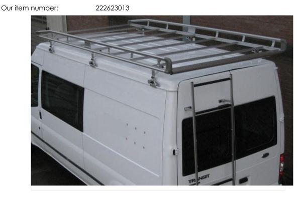
Alu Rack - the unique aerodynamic aluminum roof rack is the first choice for any truck model. Minimum weight with maximum strength in aerodynamic design. The Alurack includes a complete system. The cross rails of the carrier basket can be added as options. The system is designed for a load up to 150 kg (Note nevertheless the maximum roof load of the vehicle manufacturer). For the Ford Transit model 2006 with long wheelbase 3750 cm, extended rear and high roof.
