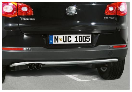
Side protection bar made from high quality hand polish stainless steel - for a beautifull mirror finish and a exceptional corrosion protection. The computer-aided development provides a perfect fit and design. Comes with TÜV approval documents. Included fitting instruction for an easy fitting in 30-60 minutes. For the VW Tiguan model 07/2011.
