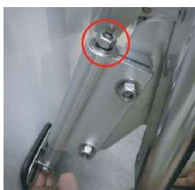
B. Secure the "door lower bracket" (2) with the washer and nut (by hand) so that the "door lower bracket" (2) remains clipped around the door.
