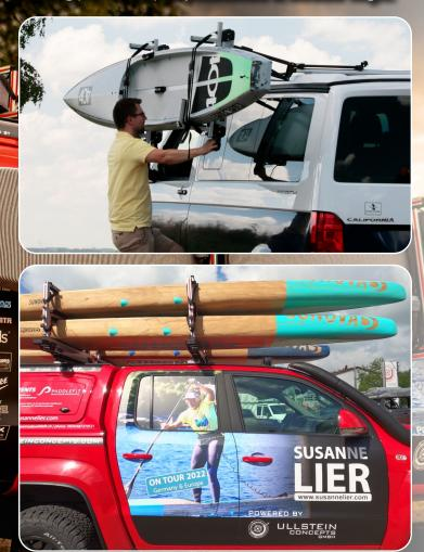
Gas springs reduce the weight of the board by up to 18 kg when lifting and lowering the SUP Rack. If the SUP Rack is not in use, it can be disassembled easily by removing only one locking bolt, leaving only the mounting plate of the cross bars.
